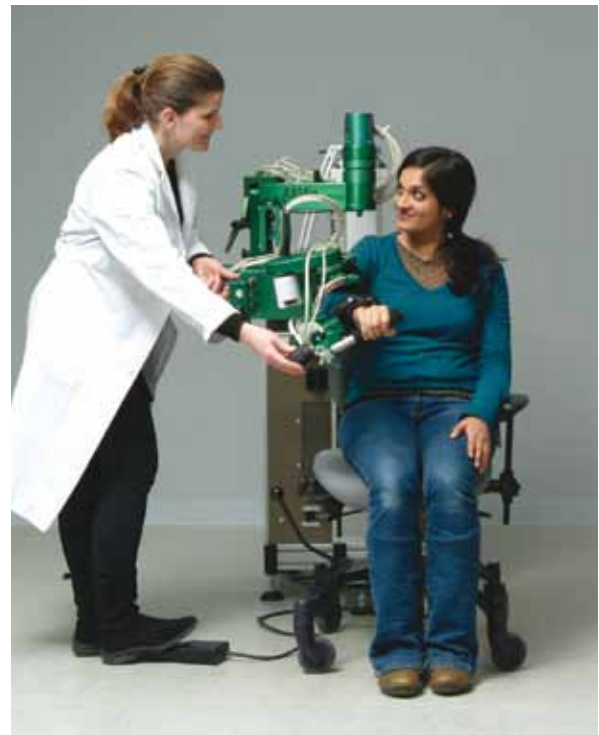
Case-study of the robotic arm therapy system ARMin (T. Nef, M. Guidali, R. Riener, Applied Bionics and Biomechanics , 2009).
