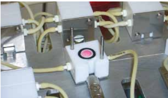
Perfusion chamber for the culture of intervertebral disc cells enhances tissue growth through increased solute transport.
